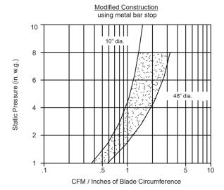
Leakage results shown are based on tests using various damper sizes. The shaded area between the graph lines indicate normal expected leakage range for a standard damper operating conditions and sizes.
